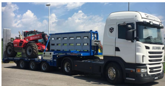
Figure 4 - Truck for weighbridge verification, total weight 40 t, equipped with a set of 500 kg and 1000 kg weights that can be handled by a pallet truck
