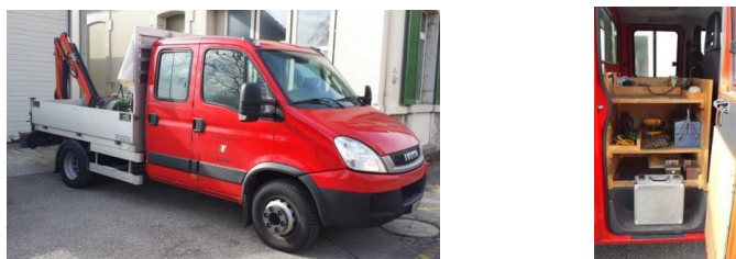
Figure 3 - Van for the verification of medium-size weighing instruments, equipped with a crane, 2-4 racks containing 20 kg weights, a set of 500 kg weights, sets of additional weights, and various accessories
